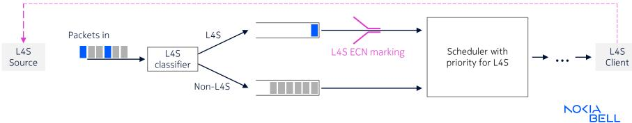
L4S enables scalability in low-latency service offerings Through fast rate-adaptation, while safeguarding QoE
