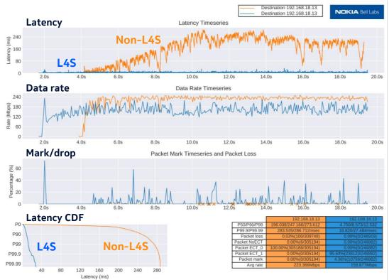
**Note:** Measurement on Nokia WiFi Beacon6 with reduced channel power and spectrum (20MHz)
